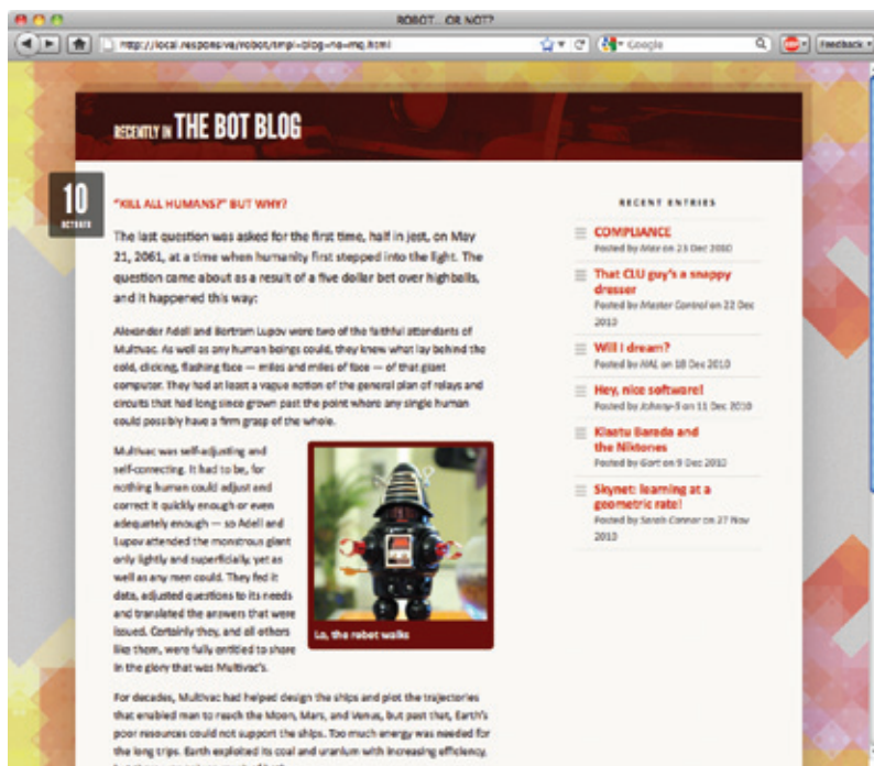
FIG 3.3: Just by including max-width: 100% , we've prevented our image from escaping its flexible container. On a related note, I love max-width: 100% .
